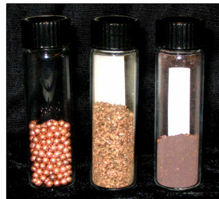
Copper produced as bright plating (left), bright flake (center) and dendrites (right) with Eltron's electrowinning technology.
