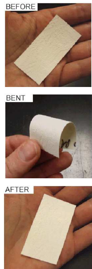
Figure 1. Photographs of ceramic coated polyethylene terephthalate (Mylar ® ) flexible substrate showing no cracking or delamination during 180° bending.
