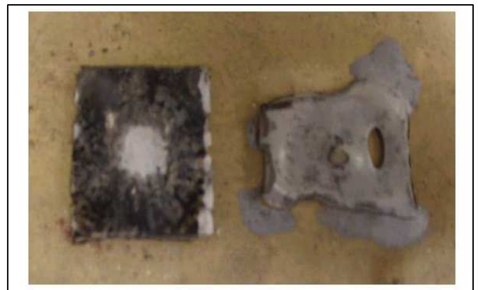
Figure 3. Refractory paint coated square (left) and uncoated square (right) of high density polyethylene after exposure to direct flame of a propane torch for 20 seconds, at a distance of 1 inch.
